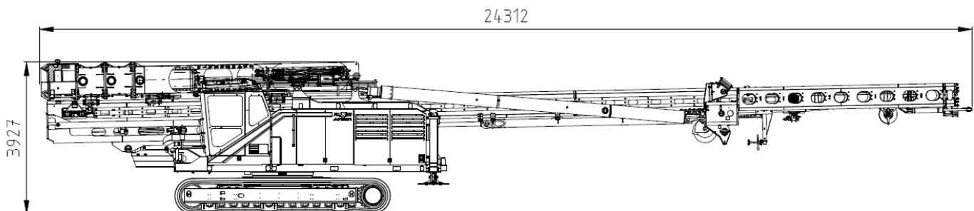
PMx28 transport dimensions with longest available leader configuration (Hydraulic Impact Hammer SHK 110-9).
